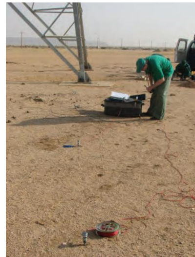
Figure3. Measurement of soil resistivity in the vicinity of the tower no. 31.
